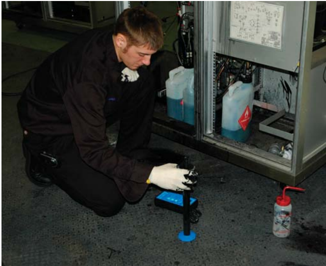
Justin Kreuger of A2N, Inc. using the Hydramotion Viscolite® to check ink viscosity on an industrial inkjet printer
